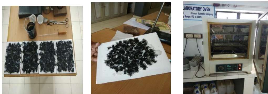
Fig 2.5 Grafting MWCNT-F on CF Surface
